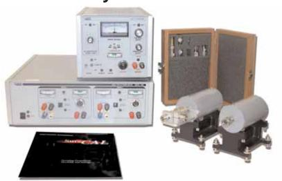
The System IIA can be used manually via front panel controls. The task of calibrating power sensors is fully automated by the SureCal calibration software. **Precision RF Power Source**
